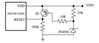
Fig. 15 Circuit 1 for the residue voltage protection
