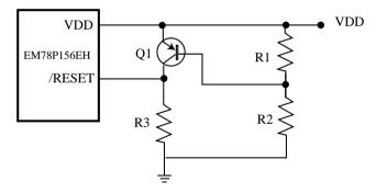
Fig. 16 Circuit 2 for the residue voltage protection
