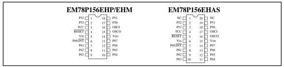
Fig. 1 Pin assignments
