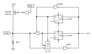
\* The Rex is 430K ohm external resistor.
