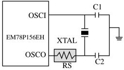
Fig. 12 Circuit for Crystal/Resonator
