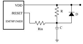
Fig. 14 External Power-up Reset Circuit
