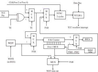
Fig. 5 Block diagram of TCC and WDT
