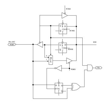
\*Pull-high (down) and open-drain are not shown in the figure.
