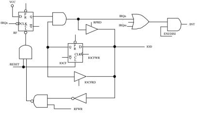
Fig. 10 Interrupt input circuit
